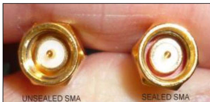
Figure 3 - Unsealed vs Sealed SMA Connectors
