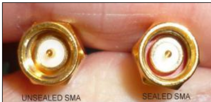
Figure 3 - Unsealed vs Sealed SMA Connectors
