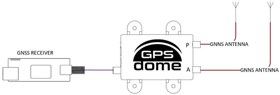
Figure 4 – GPSdome 1.03 - EPS - Operational Diagram
